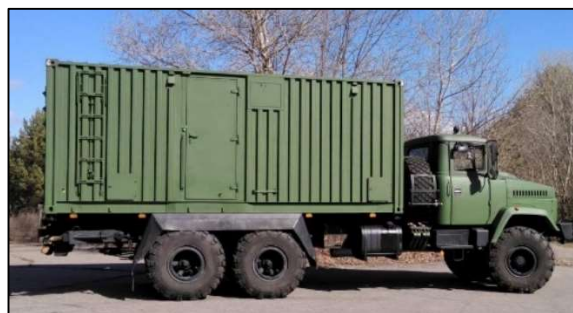
Figure 6 – Mobile bath and laundry module
