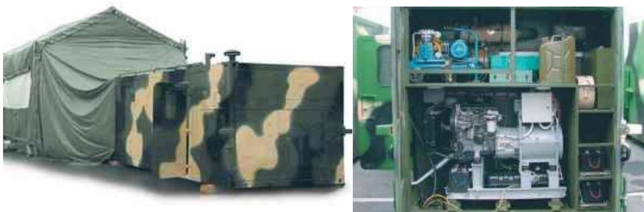
Figure 2 – Workshop for the repair of technical means of the food service RMTP-9
