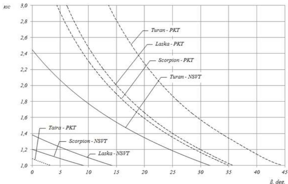
Figure 4 – Dependence of the relative stability factor on the angle of inclination for some combinations of unmanned platforms with small arms samples at  $h_e = 1,3$  m,  $\Theta_0 = \beta$
