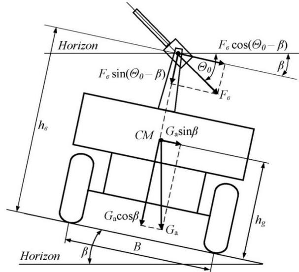
Figure 2 – Diagram of the forces and moments acting on the centre of mass of the vehicle, located on a surface with a lateral slope, when firing a weapon
