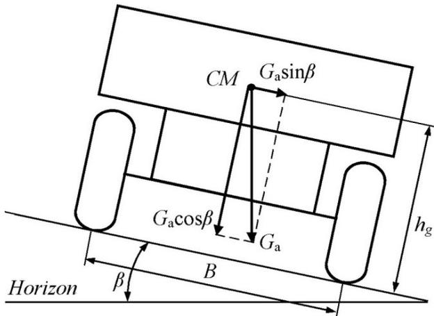
Figure 1 – Diagram of forces and moments acting on the centre of mass of a vehicle, located on a surface with a lateral slope
