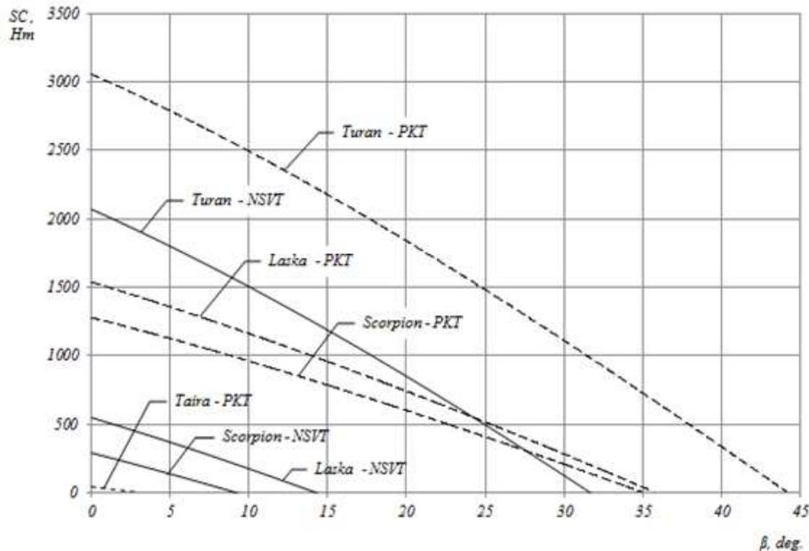
Figure 3 – Dependence of the stability coefficient on the angle of inclination for some combinations of unmanned platforms with small samples at  $h_e = 1.3$  m,  $\theta_0 = \beta$
